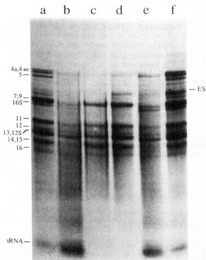
Fig. 1. Electrophoretic patterns in agarose- CH_3HgOH slab gels of liver mitochondrial RNA synthesized in isolated organelles from control (lanes a-c) and ethanol-fed (lanes d-f) rats. Lanes a and f, total RNA; lanes b and e, oligo(dT)-cellulose-unbound RNA; lanes c and d, oligo(dT)-cellulose-bound RNA. Equivalent amounts of material were run in the lanes that correspond to the same RNA fraction of control and ethanol mitochondria.
